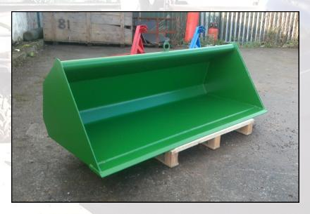
All our buckets are manufactured with 150mm x 20mm (6" x 3/4") 270HB Boron cuttings edges, 10mm leading edges on the side plates and wear ribs on the floor as standard.
