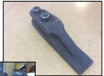
Bolt on teeth and side cutters for mini and midi excavator buckets inc. Kubota , JCB and MF style teeth
