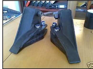
Bolt on teeth and side cutters for mini and midi excavator buckets inc. Kubota , JCB and MF style teeth
